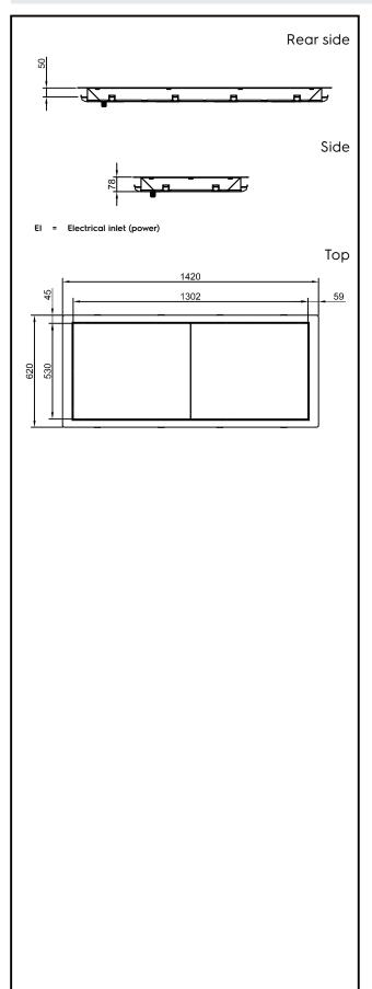
Drop-In Drop-in tempered glass top (4 GN container capacity)
