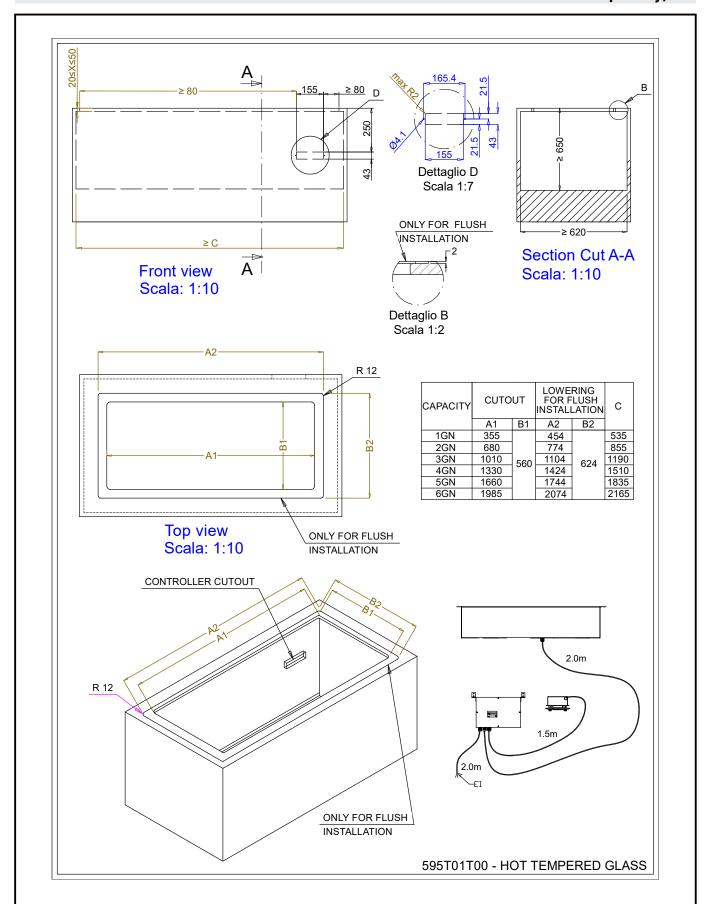
Drop-in tempered glass top (4 GN container capacity)
